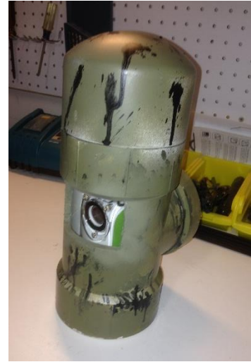
Figure 2. Custom 4" PVC housing
