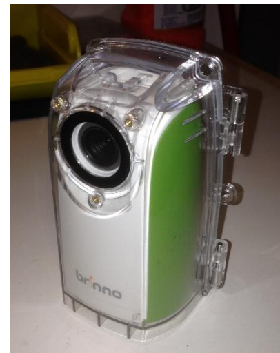
Figure 1. Brinno TLC 200 TimeLapse HD Video Camera inside ATH110 Weather Resistant Housing
